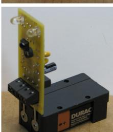
Snap board onto a 9 VDC battery. When first connected the LEDs may illuminate then shut off after a few seconds.
